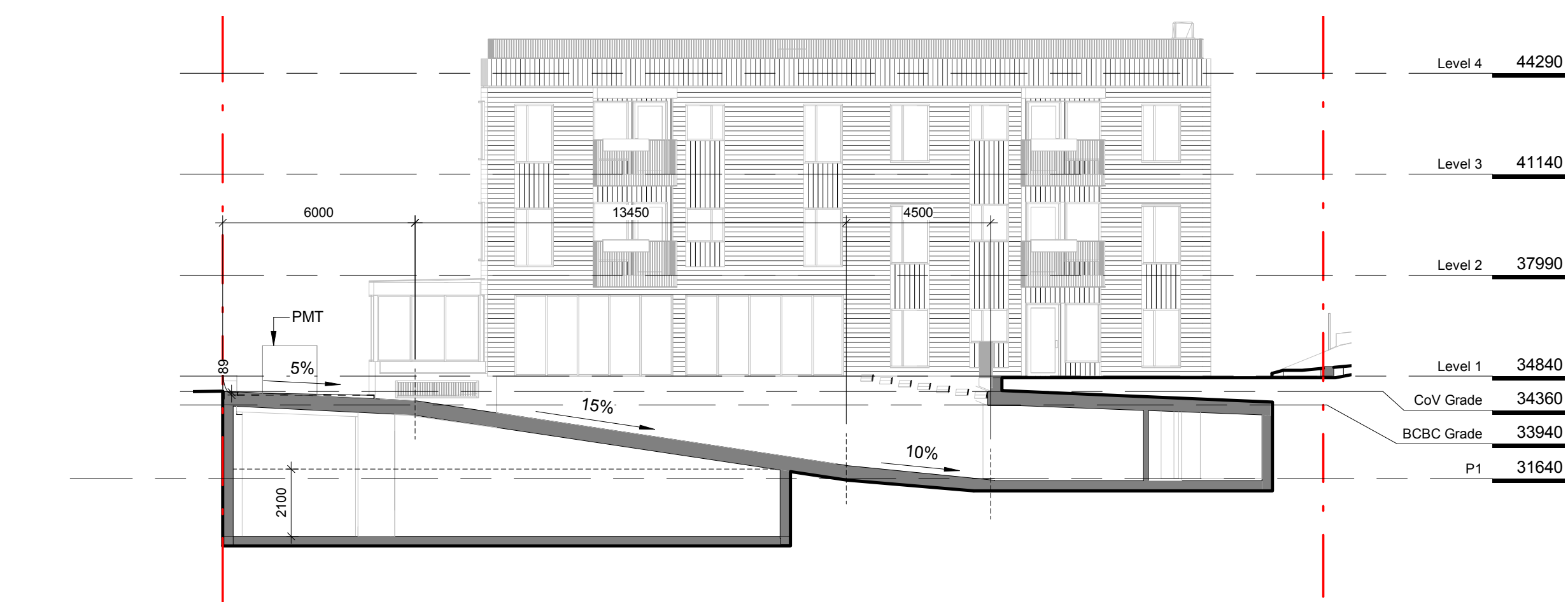
3 Parking Ramp Section SCALE = 1 : 150
