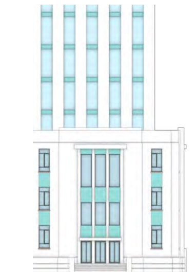
Step 2. Articulate the horizontals using recessed cladding elements, referencing the language of the existing to delineate floors.
