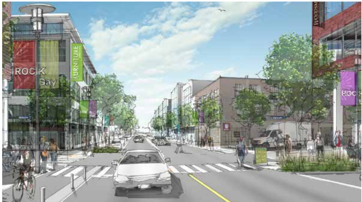
Figure 15: Concept drawing showing future vision for Bridge Street, with protected bicycle lanes, new crossing Hillside Avenue, street trees, and new buildings with industrial at grade as well as spaces for employees to gather.
