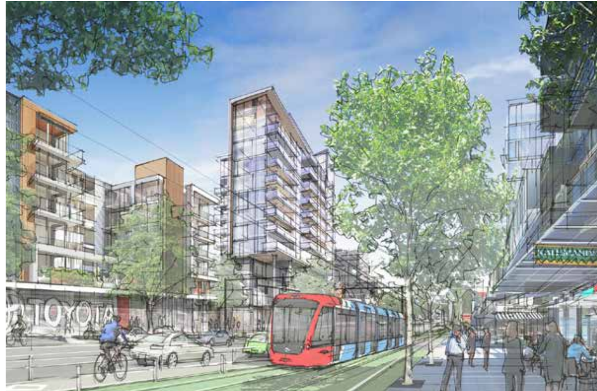
Figure 9: Concept drawing showing an example of a frequent transit route through a Town Centre, with enhanced sidewalk and protected bicycle lanes framed in by tall buildings. In this example, Light Rail Transit (LRT) is shown with tracks along the side of the right-of-way, although centre lane is another common case for LRT.
