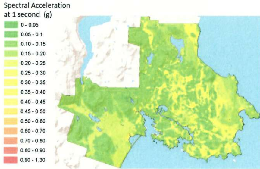
Figure 7: Ground Motion Intensity (1 Second Spectral Acceleration) Expected from the M = 7 Inslab Earthquake Scenario
