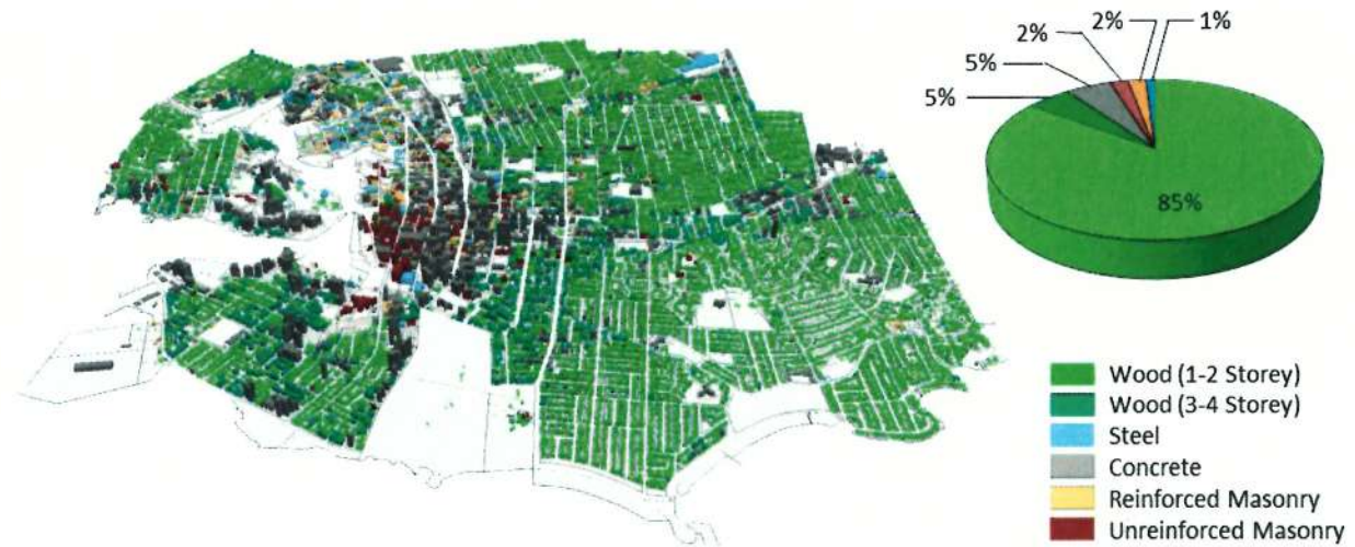
Figure 12: Distribution of City of Victoria Buildings Based on Construction Type
