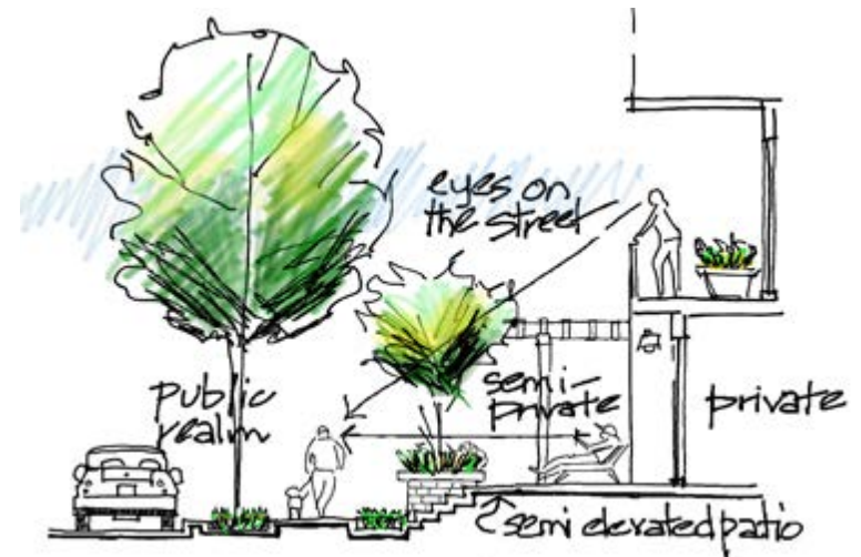
Diagram showing incorporation of entries to individual ground floor units that are accessible and clearly visible from the fronting street.
