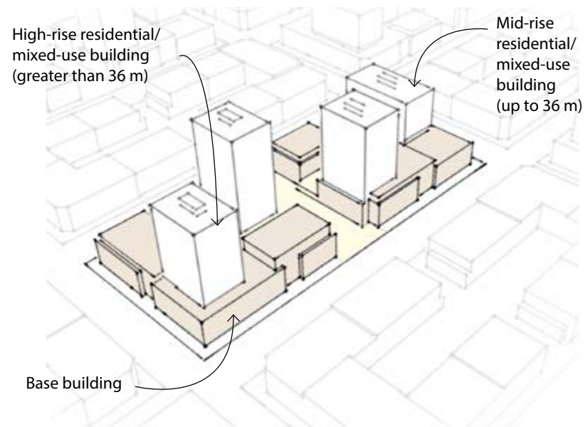
Diagram illustrating accommodation of mid and high rise buildings within a perimeter-block form of development.
