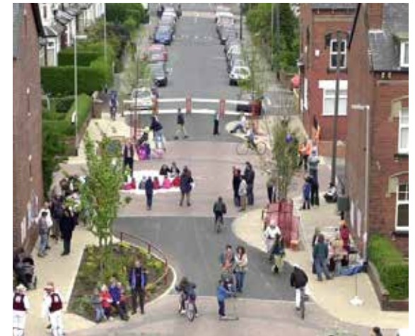
Figure 18. Example of living streets using woonerf street design feature in United Kingdom (image credit: methleys.headstogether.org)
