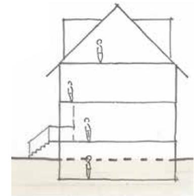
Figure 50. Example of one way to achieve a 2.5 storey infill building with a daylight basement (See policy 8.11.9).
