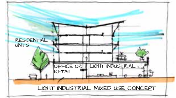
Figure 36. Illustrative diagram of a mixed use development with light industrial uses at grade
